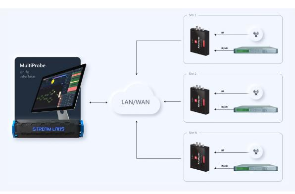
Above is an example where an operator may use multiple TS analyzers in different parts of their network to monitor and aggregate data and analytics as well as provide alarm services to an upper level Broadcast monitoring system such as Multiprobe.
